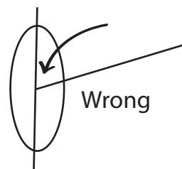
In the example above the axes are incorrect because the major axis is not at a right angle (90 degree angle).
